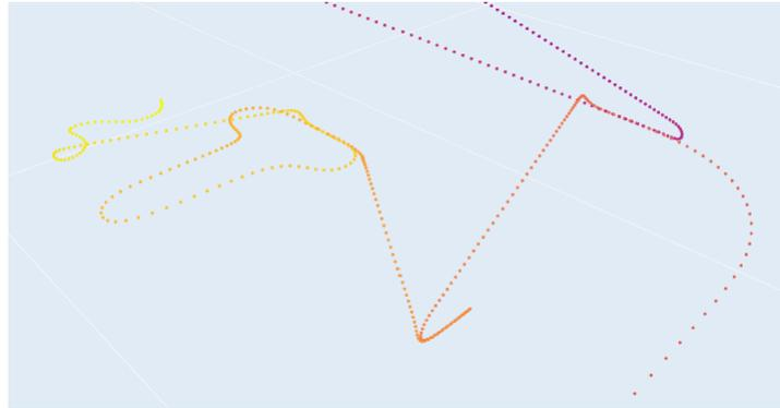
Figure 19: MAXL uses basis spline interpolation as a generic intermediate representation for motion. In this figure, I render a subset of spline control points that were generated by MAXL to stream to motors during a print job.
